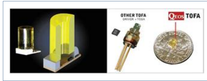
(left) The QEOS Transmitter Optical Full Assembly™ (TOFA). (right) Size comparison between a current optical transmitter solution and the QEOS TOFA
